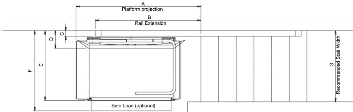
Note: Dimension F only applies at lower landing when the side load ramp is in the open position.
