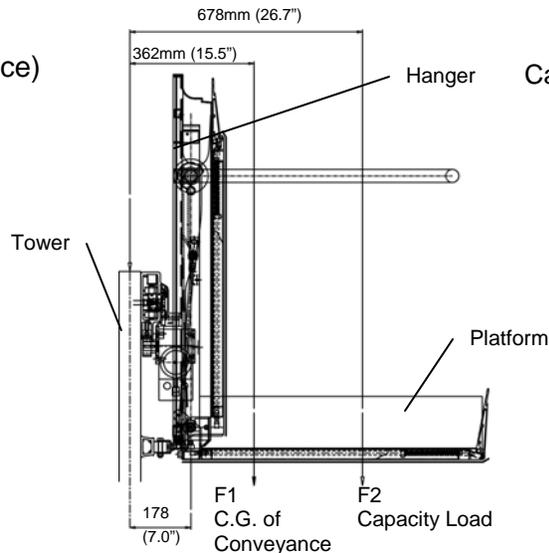
Loading Calculations are based on a 1220 / 1250 platform
