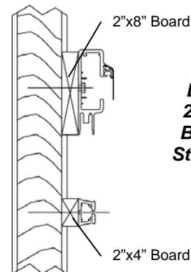
**Direct Mount to 2"x8" and 2"x4" Boards on Wood Stud or Thin Block Wall**
